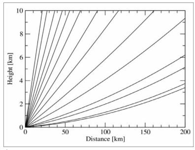
Figure 1: volume Coverage Pattern of both KNMI radars with 14 elevation angles: 0.3, 0.4, 0.8, 1.1, 2, 3, 4.5, 6, 7, 10, 12, 15, 20, and 25°.
